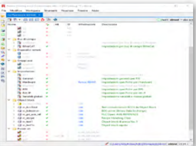
Machine Configurator It allows to describe an axis, a group of axes, kinematics, a power set etc.
